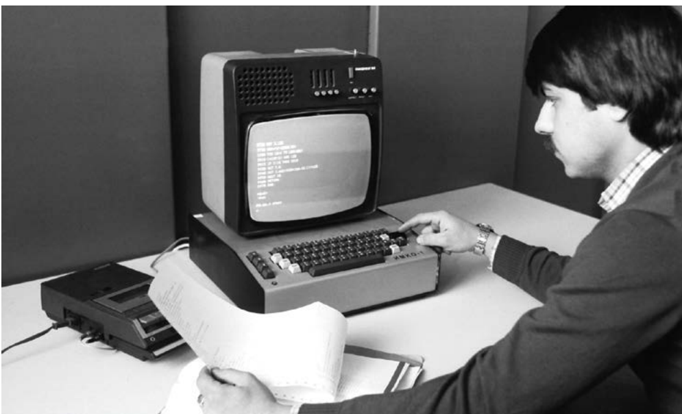
Sofia, January 19, 1982. IMKO-1, the first Bulgarian personal computer created by specialists at the Institute of Technical Cybernetics and Robotics with BAS. Based on the Intel 8080 microprocessor on one big-printed circuit board, the computer has a keyboard for manual data entry. The necessary information is displayed on the screen of a regular black-and-white television, and a regular cassette player serves as peripheral memory. The computer can be connected to print and other devices.
